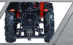
HYDRAULIC LIFTING CAPACITY 500KG
